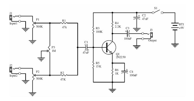
This is a classic signal mixer that is used for audio purpose. VR1 & VR2 are inputs audio volume controlers and VR3 is used to control the balance between Input1 and Input2.
